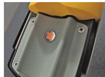
The TruTouch 2500 transmits safe, non-invasive near infra-red (NIR) light into the skin via contact with an optical touch pad. It then collects a portion of the light reflected back by the skin and analyzes it to determine tissue alcohol concentration and verify user identity
